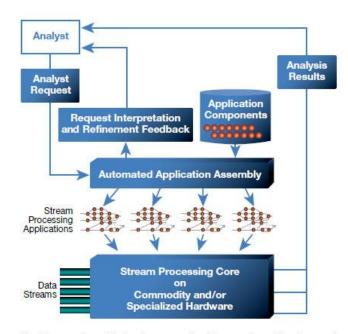
The diagram shows the business user (top left corner), and how the user's analysis request is converted into a stream processing application, deployed into the compute environment as a distributed stream processing job. It also shows how the analysis results are returned, rendered as a dynamic mashup and presented to the business user. (Credit: IBM)
